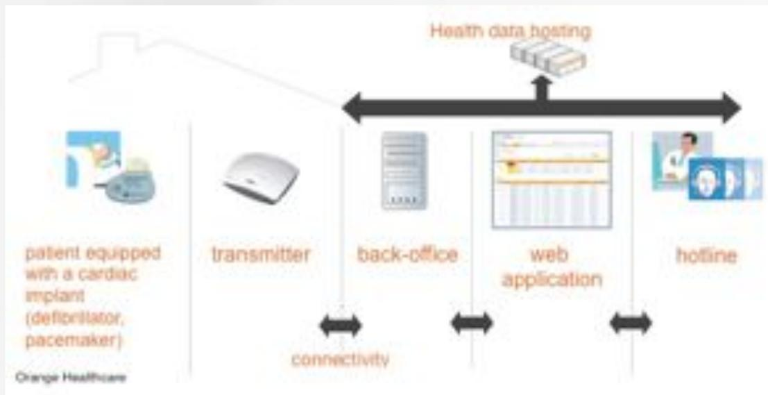
The device is not connected to a mobile or GSM (Global System for Mobile Communications) network. The implant is entirely autonomous. The objective of the network is to receive information daily from the implant and store it. It can be sent, if necessary, to the physician in charge. Rhythmology and cardiac remote management are growing fields in France.
